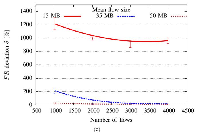
Fig. 5. FR drop duration in FAN with standard RED (a), RED with decreasing probability (b), and FAN with limitation mechanism (c) with respect to various traffic patterns.
