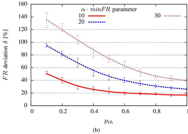
Fig. 4. FR deviation in FAN with standard RED (a) and RED with decreasing probability (b) with respect to various traffic patterns.
