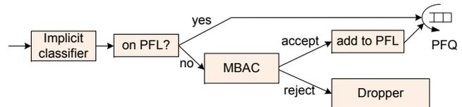
Fig. 1. The principle of FAN operations
