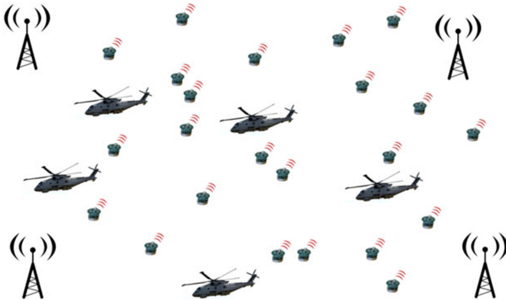
Figure 3. The network architecture: base stations, actuators (these can be UAVs or helicopters) and sensors deployed in a monitored area. Sensors are communicating with base stations by multiple hops. Actuators are assumed to have stronger radio transceivers and can communicate directly.
